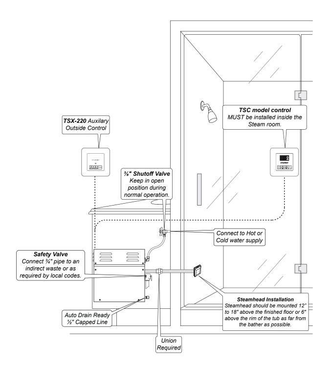
Steam Outlet Pipe - Use a ¾" Copper or Brass pipe.
