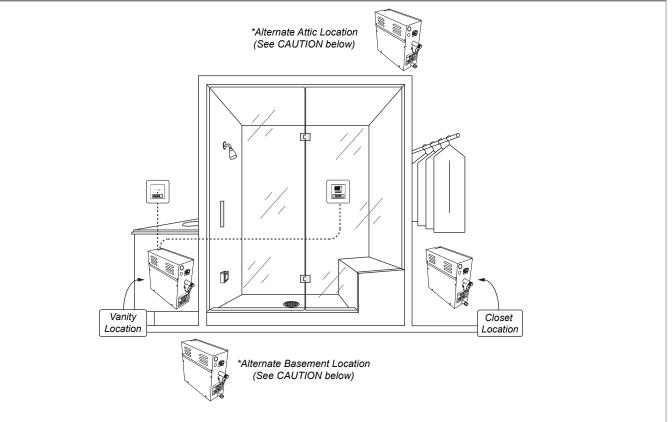
\*CAUTION: Steam generators must NOT be installed outdoors, in moist, humid areas, in areas prone to freezing, or extreme heat such as an unventilated attic. To do so will void the warranty.
