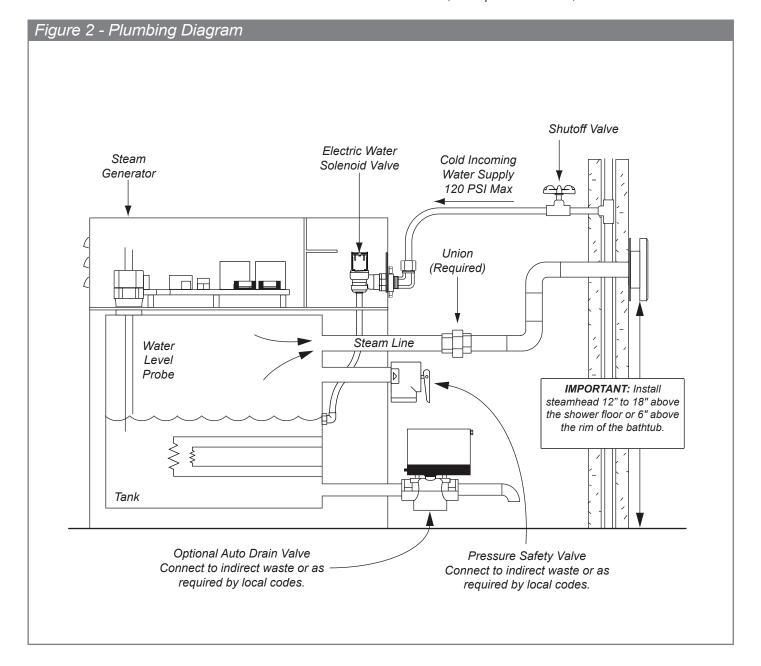
Figure 4 - Typical Installation
