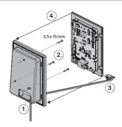
Figure 5 - Opening the Power Unit Cover and Mounting the Unit to a Wall
