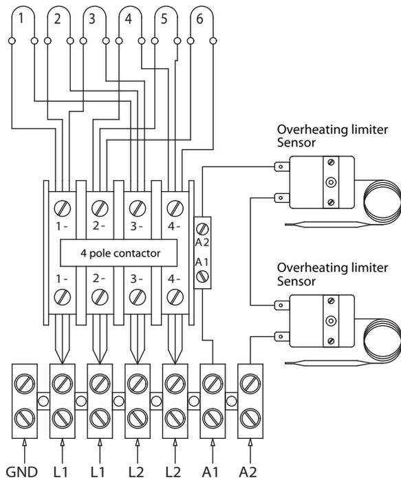
Figure 9 - SMS-100-3, SMS-125-3, and SMS-145-3
